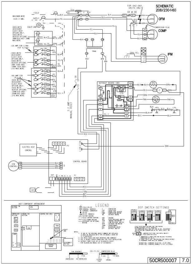
Fig. 15 - Wiring Schematics-50CR Single Phase
